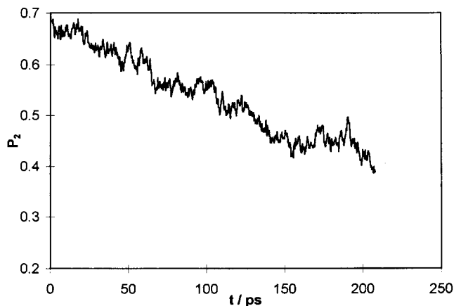
Figure 9. Order parameter ( P_2 ) variation after switching off the electrostatic interactions in the nematic state at 330 K.
